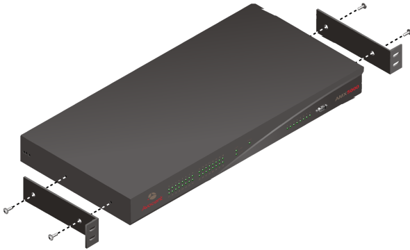
Figure 2.4: AMX5000 Switch Rack Mounting Diagram
