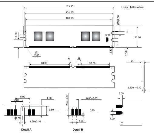
Figure 1: KVR400D2N3/256 240-Pin DIMM
