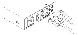
5. Locate the power cord that came with your SwitchView OSD unit. Plug it into the IEC power connector on the SwitchView OSD. Make sure that the SwitchView OSD power switch is off, then plug the other end of the power cord into an appropriate AC wall outlet. This outlet must be near the equipment and easily accessible to allow for unplugging prior to any servicing of the unit.
