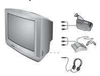
Depending on the versions, the connectors are located on the front (sometimes under a flap) or on the right-hand side of the TV set. Make the connections as shown opposite. With the (a) key, select AV / S-VHS.
