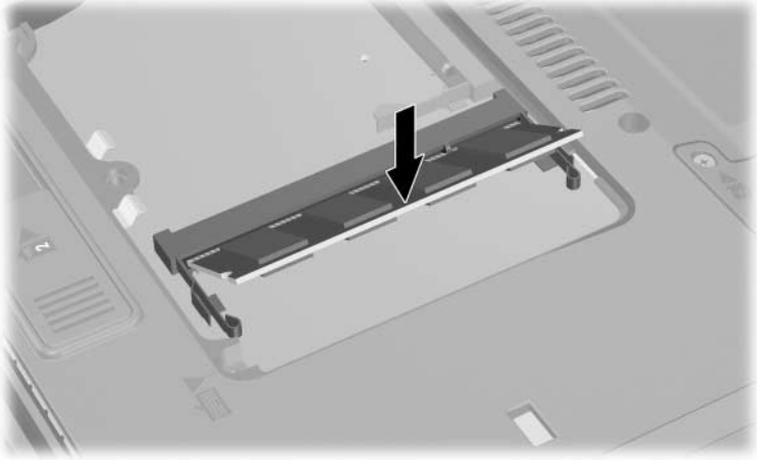
10. Replace the memory module cover **1** and tighten the memory module cover screw **2**.
