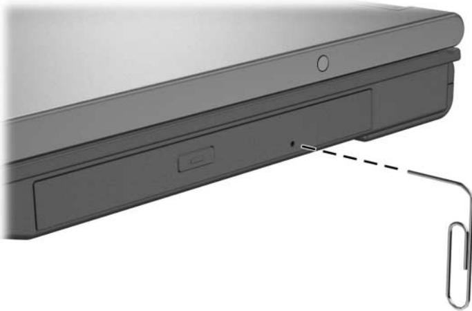
2. Press gently on the paper clip until the media tray is released, and then pull out the tray until it is fully extended.
