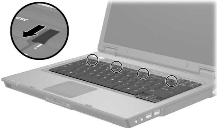
11. Gently lift the top edge of the keyboard and tilt the keyboard over until it rests on the palm rest of the notebook.
