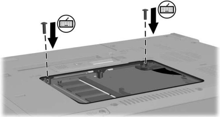
16. Replace the memory module cover **1** and the memory module cover screw **2**.
