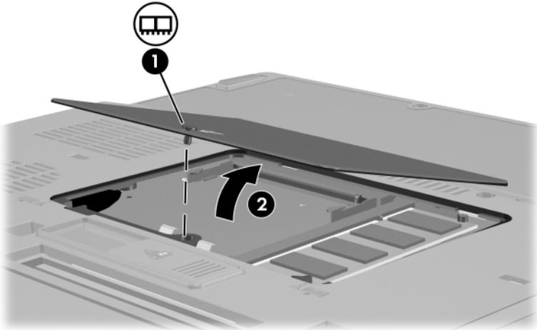
8. If there is a memory module in the expansion memory module slot, remove it:
