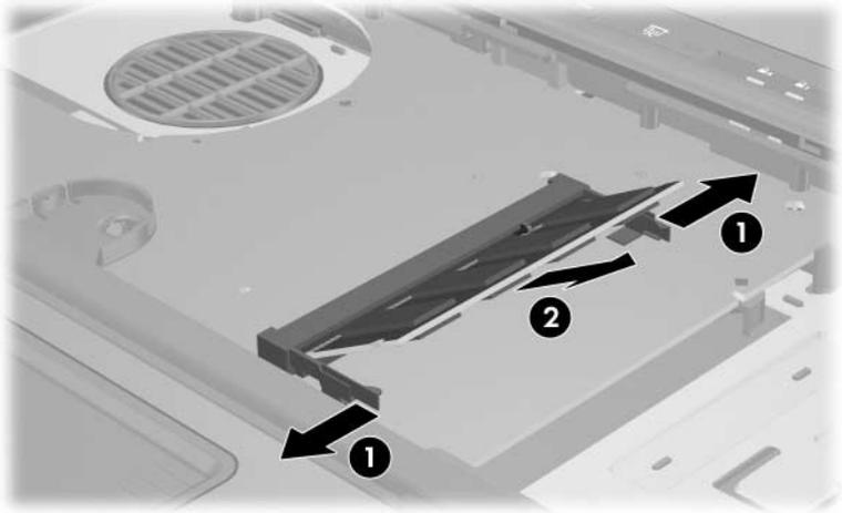
13. Insert the new memory module into the memory module slot:
