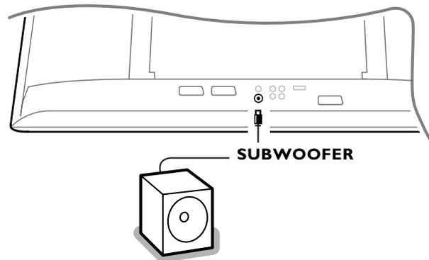
To enhance the sound reproduction of your TV you can connect an externally powered subwoofer (between 20 and 250 Hz).
