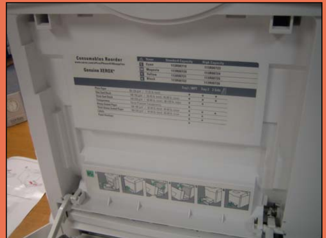
A convenient reference chart above the bypass tray provides helpful toner replacement information and maximum paper capacity for different media types.
