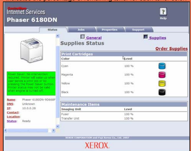
The General Status page displays the status of paper drawers (full or empty), and a count of total printed pages. The Supplies Status page indicates the percentage of remaining toner for each toner color.
