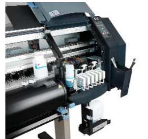
Cleaning station and self-contained tools
