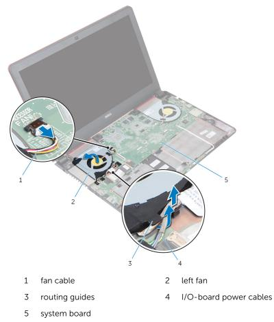
4 Disconnect the right-fan cable from the system board.
