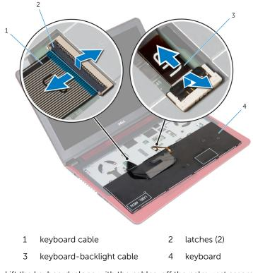
**5** Lift the keyboard, along with the cables, off the palm-rest assembly.
