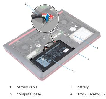
**3** Using the pull tab, lift the battery, along with its cable, out of the computer base.
