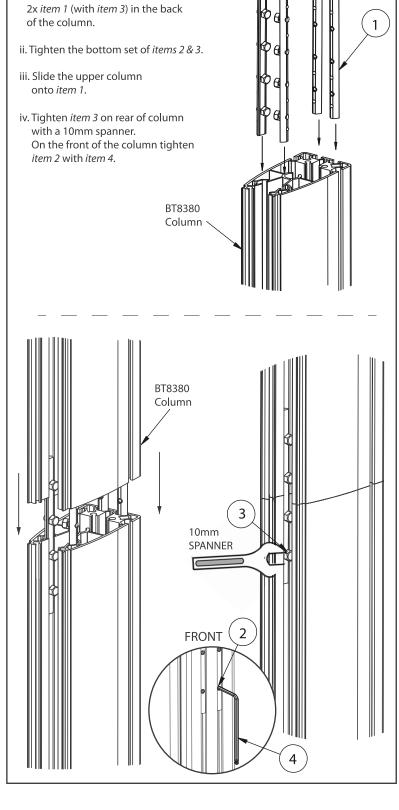
**DESIGNED TO CONNECT TWO BT8380 VERTICAL COLUMNS**
