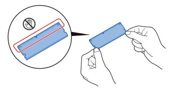
To protect electronic parts, discharge static electricity from your body by touching a water pipe (faucet) or other large metal object before handling the memory modules. Or, wear an antistatic wrist strap, if possible, when you install the memory modules.
