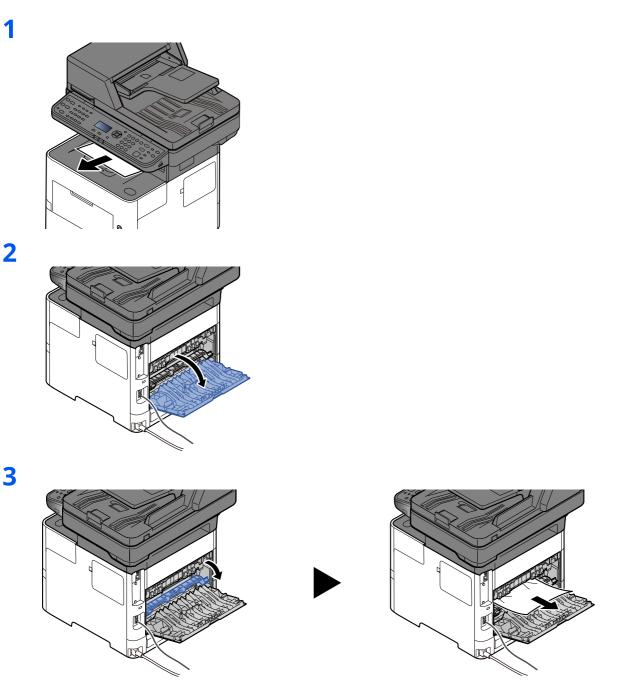
If you cannot find a paper jam, try checking inside the rear of the machine.
