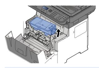
**NOTE** When removing the toner container from the machine, lift up the right hand side first.
