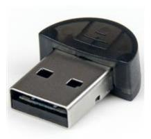
The USBBT2EDR2 USB to Class 2 Bluetooth Adapter with EDR is a micro-sized adapter that adds Bluetooth capabilities to a computer through an available USB port, which enables you to connect to devices wirelessly, at ranges up to 10m (32ft) while consuming minimal power.
