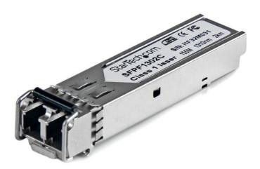
The SFPF1302C is a Cisco GLC-FE-100FX compatible fiber transceiver module that has been designed, programmed and tested to work with Cisco® brand switches and routers. It delivers dependable 100 Mb connectivity over fiber cable, for 100BASE-FX compliant networks, with a maximum distance of up to 2 km (1.2 mi).
