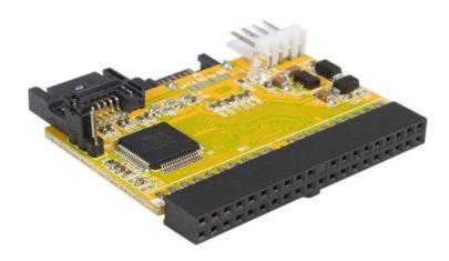
This IDE to SATA Drive Adapter Kit offers a simple way to install Serial ATA hard drives using an available IDE port - a cost-effective solution for using newer SATA drives on a legacy computer or a computer with all SATA connections already in use.
