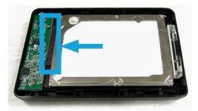
4. Align the hooks on the top panel with the groves on the Base of the enclosure and slide the top panel back into place.
