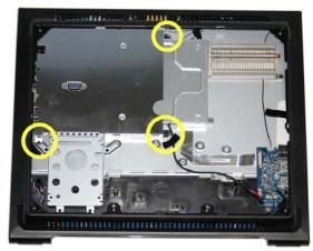
(5) As the next step, remove the large electromagnetic shielding (EMI cover). This metal sheet is fixed by three cross-head screws.
