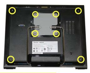
(3) Loosen the four cross-head screws (or Phillips screws) to remove the stand. Remove the four cross-head screws that fix the case cover.
