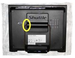
(2) Disconnect the device from the mains and put it on a soft base with the display facing downward and fold the stand vertically upward. Next, carefully remove the cap with the Shuttle logo that is clicked into place by six hooks. The cap can be loosened using a plastic card.
