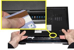
(4) The case cover is clicked into place by several hooks. At the bottom of the case is a notch that can be used to lever the case cover out of place by carefully using a screwdriver or plastic card. Be sure to apply only little force in order not to break the hooks.
