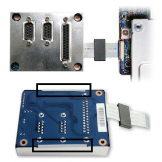
(10) Mount the electromagnetic shield of the COM/LPT adapter for which the hexagon screws need to be removed temporarily. Note: The electromagnetic shield must be attached to board so that the metal fixations of the shield clasp the board. Please connect the adapter with the mainboard afterwards. Make sure to have the cable and ferrite core aligned properly so that the electromagnetic shield is not damaged during further assembly.
