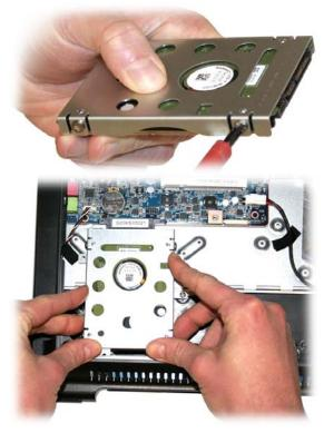
(7) Please insert a 2.5 inch S-ATA hard disk with the connectors facing towards the metal sheet into the drive cage. Please then fix the hard disk with four screws and carefully push it in afterwards to connect it. Please fix the drive cage with four screws.
