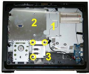
(11) Please re-mount the little (1) and the large (2) electromagnetic shield. Please affix the COM/LPT adapter (3) with three screws.
