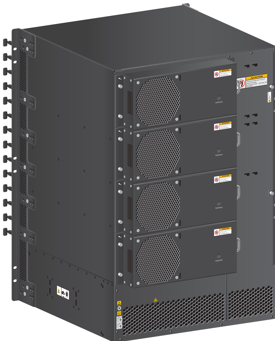
Figure 3-6 S9712 chassis (rear view)
