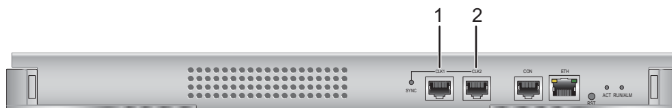
Figure 6-24 BITS ports of the LE0D00CKMA00 on the MPU panel
