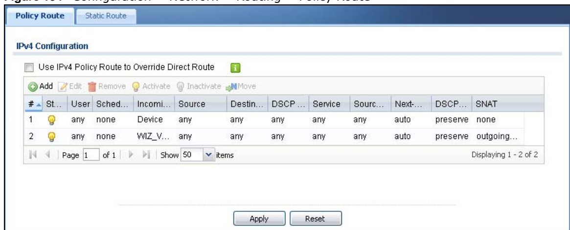
Figure 134 Configuration > Network > Routing > Policy Route
