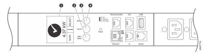
**NOTE:** Your Rack PDU is configured so the display backlight turns off after 10 minutes of inactivity. The backlight can be turned on by depressing any button below the display.
