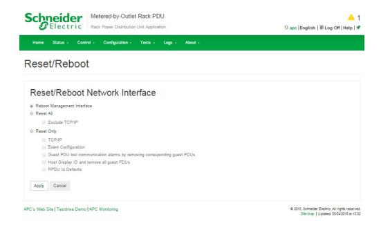
Reset All: Clear the Exclude TCP/IP checkbox to reset all configuration values; mark the Exclude TCP/IP checkbox to reset all values except TCP/IP.
