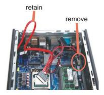
Please connect the 3.5" HDD power connectors to PW1 (3-pin) and PW2 (4-pin), then proceed to install the CPU thermal module.
