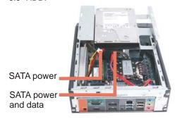
Slide the rack back into the chassis and refasten four screws.
