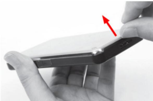
3. Place the 2.5" SATA drive into the bay (label side down) and slide the drive onto the SATA connector. Make sure the drive is fully seated.
