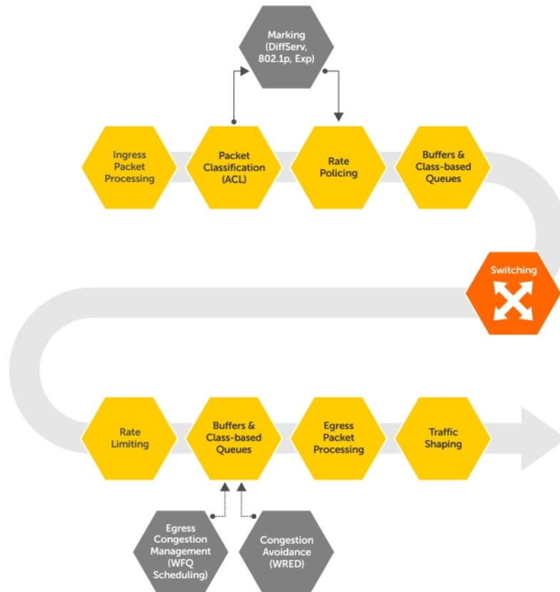
Figure 100. Dell EMC Networking QoS Architecture
