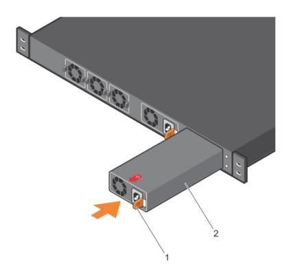
Figure 12. PSU installation
