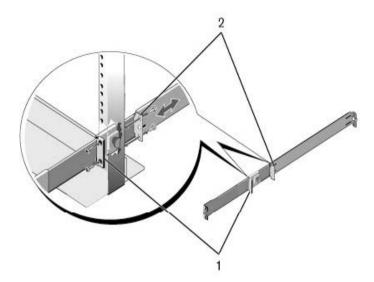
Figure 7. Two-post center-mount configuration
