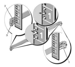
Figure 5. 1U tool-less configuration
