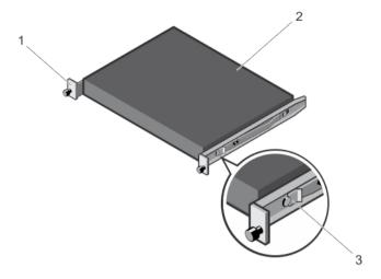
Figure 9. Switch rails attachment
