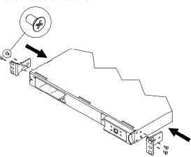
**5** Secure clip nuts to the rack, and attach brackets with provided screws.
