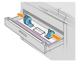
5. Place the roll into the drawer between the hubs, with the paper edge as shown.
