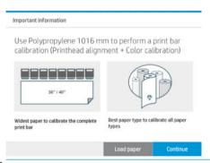
NOTE: You are highly recommended to use HP Production Matte Polypropylene, 40 in (1016mm) wide, to calibrate the print bar.
