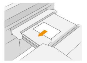
4. Move the tray to the center. The insertion rail on the table can be slid into the best position for the document you are inserting.
