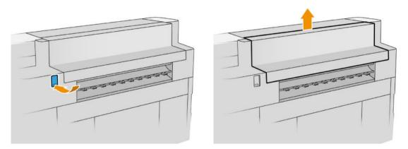
2. Remove the high-capacity stacker. You can pull the stacker by the beam at the rear of the tray.
