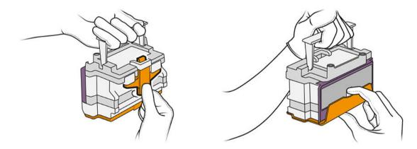
**12.** Insert the new printhead as shown below.
