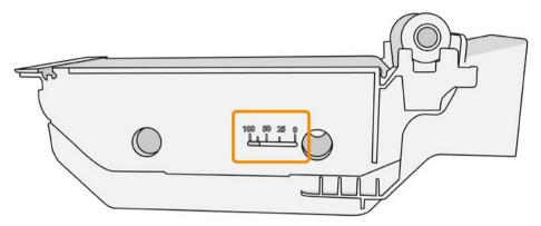
**6.** Insert the new maintenance cartridge into the slot.
