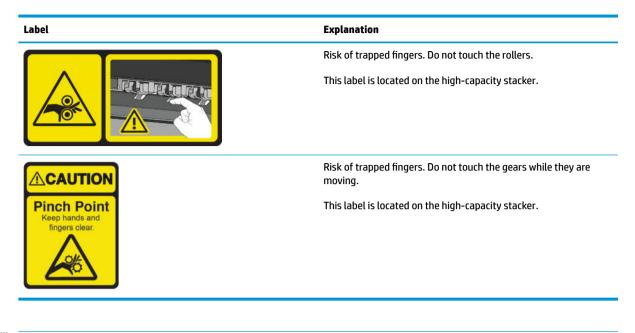
NOTE: The final label position and its size on the printer may vary slightly, but labels should always be visible and close to the potential risk area.
