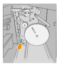
3. Rotate the tab protector to remove it.
