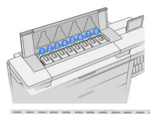
The printheads are extremely durable and do not need to be replaced every time an ink cartridge is replaced. They provide excellent results even when the ink cartridges contain a low level of ink.
