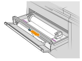
5. Remove the paper, cutting it manually if necessary.
