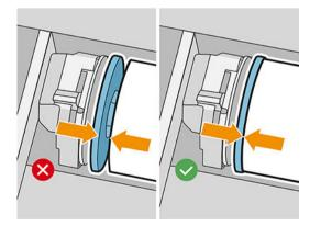
8. **Important:** Close the locking levers on the left and right hubs.
