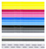
If you see defects, you should calibrate the printer by pressing **Calibrate print bar** in the optimize print quality app. You should also calibrate the printer if you are warned that a roll has a calibration pending status.
