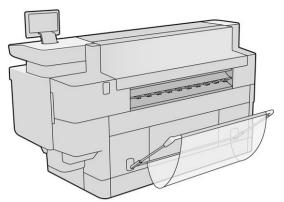
The illustration below shows the basket closed, permitting easier access to the printer (to clear printer jams, for example).
