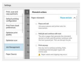
• **Pause and ask** (the most restrictive option): Printing stops until the correct paper is loaded. This option is recommended when the printer is attended. A message appears, asking what you want to do: cancel the job, print anyway, put on hold, or load paper. These options are also available in the job queue.
