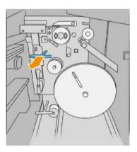
8. Open the two parts as shown so that you can pass the tab reel.
