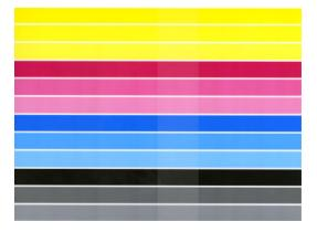
The central part of the plot indicates whether the print bar is correctly calibrated. The vertical lines indicate the boundaries of the different print elements within a printhead (die boundaries). In the horizontal gray band, no repetitive white lines or dark lines should be seen above the die boundaries. The horizontal lines of different colors should be continuous and not broken or jagged at the die boundaries; if this occurs, a printhead alignment is required.
