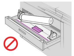
6. Slide the hubs back towards the center so that they engage with the roll.
