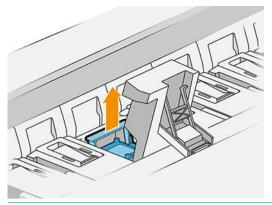
**IMPORTANT:** Printheads are fragile. Leave the printhead oriented as shown below, if you intend to use it again later. Never touch the nozzles, which could damage them. If you remove multiple printheads and intend to use them later, make sure to keep them in the right order.
