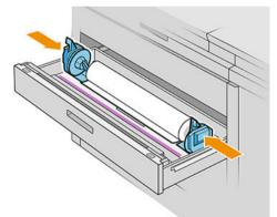
7. Ensure that the hubs are fitted tightly to the roll on both sides.
