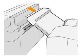
6. Push the button to raise the output module.
