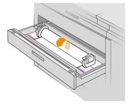
**9.** Cut off the leading edge of the paper if it has been damaged.
