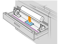
Do not load the roll at an angle, like this:
