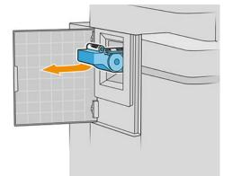
5. If you intend to insert a partially used replacement cartridge, make a note of the percentage of cloth remaining, which is shown approximately on the side of the cartridge. You will be asked for this figure later.
