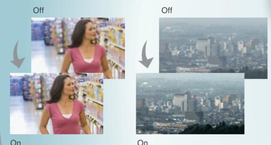
EIZO's Visibility Optimizer technology includes three functions for improving image clarity in security environments. Defog enhances images that appear hazy due to fog or snow. Low-Light Correction detects areas of the screen that are too dark and adjusts the brightness of each pixel. Outline Enhancer ensures noise is not accentuated while correcting blurred areas.
