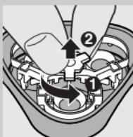
**2** Press the release button (1) and remove the shaving unit (2).
