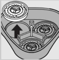
**3** Turn the wheel anticlockwise (1) and remove the retaining frame (2).
