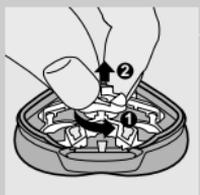
**2** Press the release button (1) and open the shaving unit (2).
