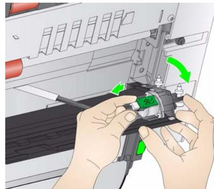
6. Install the flippable background by connecting the cable and aligning the springs on the end of the flippable background. Tighten the thumbscrews in place. *Do not over-tighten.*
