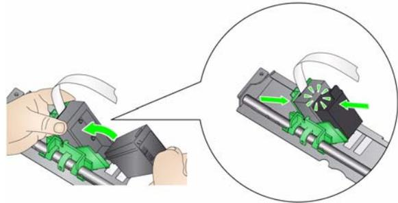
22. Rotate the printer carrier up and snap the ink cartridge in place.
