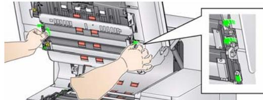
5. Unplug the connector to release and remove the flippable background.
