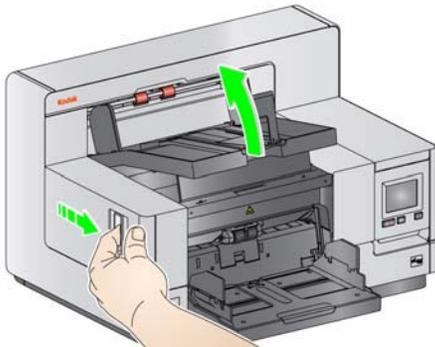
2. Loosen the thumbscrews on each end of the upper imaging guide and remove it from its position
