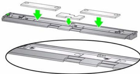
10. Install the drainage strip in place of the black strip that was removed in Step 8.
