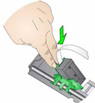
21. Snap the ink cartridge into the printer carrier as shown.
