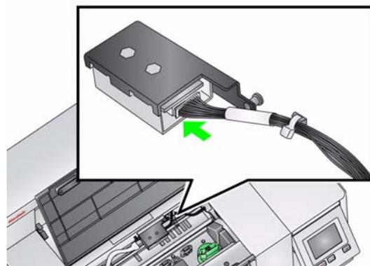
16. Snap the Enhanced Printer carrier onto the green carrier as shown.
