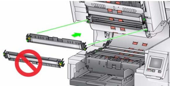
4. Loosen the upper flippable background accessory. Use the screwdriver provided to loosen all four thumbscrews.
