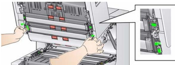
3. Install the Enhanced Printer imaging guide and tighten the screws to secure the imaging guide. *Do not over-tighten.*
