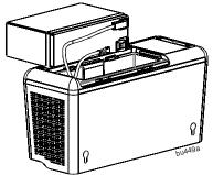
© Connect the battery cable securely to the battery terminal. It is normal for small sparks to be seen when the battery cable is connected to the battery terminal.
