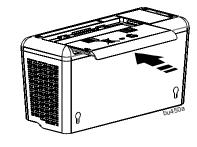
• Reinstall the battery compartment cover. Be sure that the release tabs lock into place.
