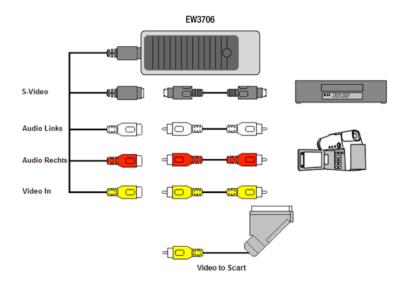
Note! The coupling plugs shown in the image are supplied with the device you wish to connect. You will therefore not find them in the packaging of the EW3706.
