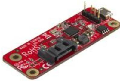
Increase the data storage capacity of your Raspberry Pi or other development board, by connecting it directly to a SATA-based drive. Perfect for custom projects and applications, this USB to SATA converter supports all models of Raspberry Pi as well as other development boards.
