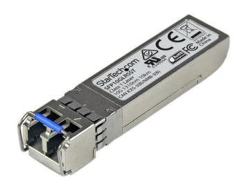
The SFP10GLRSST is a Cisco SFP-10G-LR-S compatible fiber transceiver module that has been designed, programmed and tested to work with Cisco™ brand switches and routers. It delivers dependable 10 GbE connectivity over fiber cable, for 10GBASE-LR compliant networks, with a maximum distance of up to 10 km (6.2 mi).
