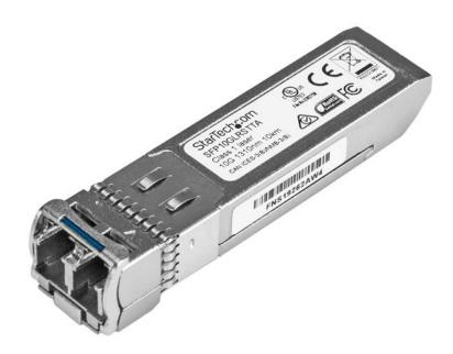
The SFP10GLRST is a TAA compliant Cisco SFP-10G-LR compatible fiber transceiver module that has been designed, programmed and tested to work with  $Cisco^{TM}$  brand switches and routers. It delivers dependable 10 GbE connectivity over fiber cable, for 10GBASE-LR compliant networks, with a maximum distance of up to 10 km (6.2 mi).
