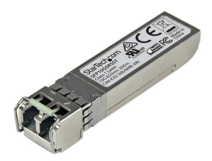
The SFP10GSRSST is a Cisco SFP-10G-SR-S compatible fiber transceiver module that has been designed, programmed and tested to work with Cisco® brand switches and routers. It delivers dependable 10GbE connectivity over fiber cable, for 10GBASE-SR compliant networks, with a maximum distance of up to 300 m (984 ft.).
