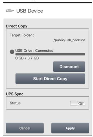
If you do, the function LED will flash as all the files on the USB device are copied to the Direct Copy folder to the LinkStation.
