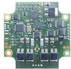
Stepper Motor Control
