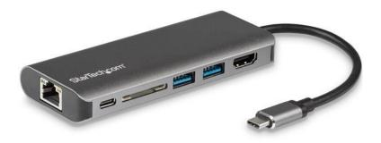
Expand the connectivity of your USB-C<sup>™</sup> enabled laptop. This USB-C multiport adapter lets you turn your laptop into a powerful workstation, virtually anywhere you go, and eliminates the hassle of carrying and connecting many different port adapters. The USB-C adapter lets you add 4K Ultra HD HDMI® video output, two USB 3.0 Type-A ports, one Gigabit Ethernet port and one SD card reader slot through your laptop's USB-C port.
