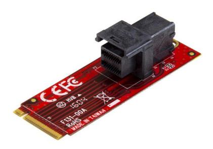
This PCI Express U.2 to M.2 adapter makes it easy to install a high-performance U.2 PCIe-NVMe SSD into your desktop PC or server and connect the drive through an M.2 PCIe x4 slot on your motherboard. By creating compatibility with newer U.2 NVMe SSDs, such as the Intel® SSD 750 series, this enterprise-class drive adapter enables you to gain faster read/write speeds and higher productivity levels for data-intensive applications.
