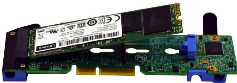
Figure 13. Dual M.2 Boot Adapter and a 128 GB M.2 drive
