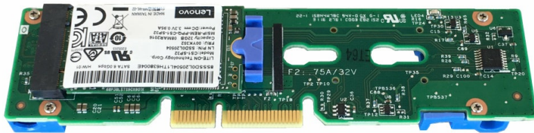
Figure 14. Single M.2 Boot Adapter and a 32 GB M.2 drive
