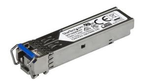
The SFP1000BXUST is an MSA compliant upstream fiber SFP transceiver which pairs with StarTech.com's SFP1000BXDST. They are designed, programmed and tested to work with 1000BASE-BX compatible MSA switches and routers. The SFP transceiver module supports a maximum distance of up to 10 km (6.2 mi) and delivers dependable 1 GbE connectivity over fiber cabling.
