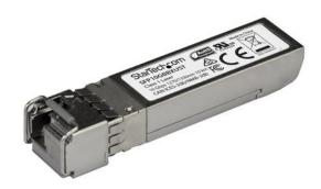
The SFP10GBBXUST is an MSA compliant upstream fiber SFP transceiver which pairs with StarTech.com's SFP10GBBXDST. They are designed, programmed and tested to work with 10GBASE-BX compatible MSA switches and routers. The SFP+ transceiver module supports a maximum distance of up to 10 km (6.2 mi) and delivers dependable 10 GbE connectivity over fiber cabling.
