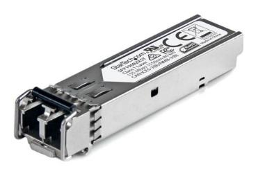
The SFP100BZXST is an MSA compliant fiber SFP transceiver that's designed, programmed and tested to work with 100BASE-ZX compatible MSA switches and routers. The SFP transceiver module supports a maximum distance of up to 80 km (49.7 mi) and delivers dependable 100 Mb Ethernet connectivity over fiber cabling.
