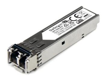
The SFP1000LHST is an MSA compliant fiber SFP transceiver that's designed, programmed and tested to work with 1000BASE-LH compatible MSA switches and routers. The SFP transceiver module supports a maximum distance of up to 40 km (24.8 mi) and delivers dependable 1 GbE connectivity over fiber cabling.
