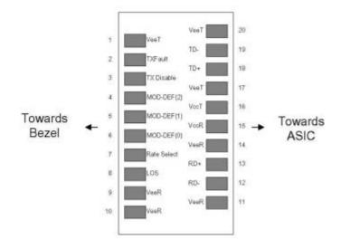
Pin-out of connector Block on Host board
