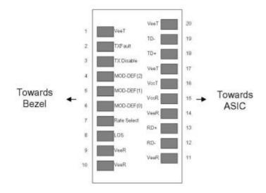
Pin-out of connector Block on Host board
