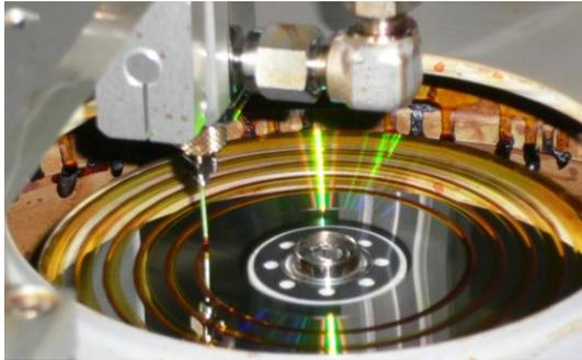
**“Spin\_coating process of LTH B-R recording layer”:**
