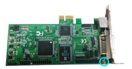
6. Re-insert the Standoff screws that you removed in step 1.
