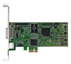
4. Line up your desired bracket so that the DVI input-port, and the A/V breakout cable input port align with the port holes. Also ensure the screw hole is aligned with the underside of the capture card.
