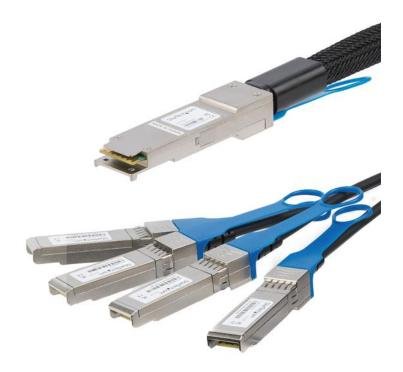
The QSFP4SFPPC2M is an MSA Compliant QSFP+ direct-attach Twinax breakout cable. It is designed, programmed and tested to bridge 40G network equipment with 10G compatible servers or routers. This passive Twin axial cable connects a single QSFP+ port to four 10G SFP+ ports and is fully hot-pluggable making upgrades and replacements seamless by minimizing network disruptions.
