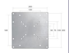
The NewStar VESA adapter, model FPMA-VESA200 allows a VESA mount with 50x50, 75x75 or 100x100 mm interface to be used with displays with VESA hole patterns of 100x200, 200x200 and 120x180 mm (JVC holepattern). Ideal when flat screen needs different VESA pattern to select wall-, desk- or ceiling mount.
